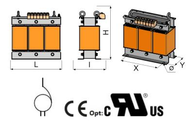
\*Dimensions are expressed in millimeters, mass in kilograms and reserves represent the ventilation space to be kept around the product for good heat dissipation. The drawing is not contractual.
