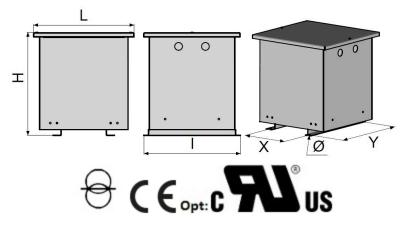
\*Dimensions are expressed in millimeters, mass in kilograms and reserves represent the ventilation space to be kept around the product for good heat dissipation. The drawing is not contractual.
