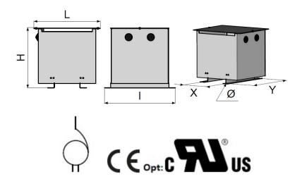
\*Dimensions are expressed in millimeters, mass in kilograms and reserves represent the ventilation space to be kept around the product for good heat dissipation. The drawing is not contractual.
